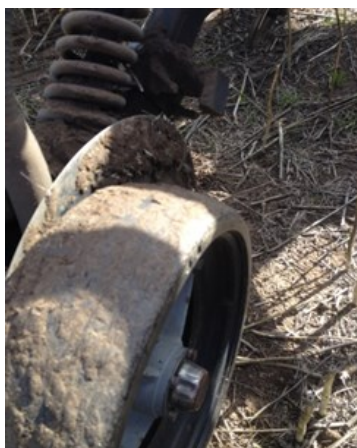
Scraper not installed - quite significant mud build up on discs.
