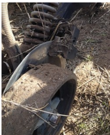
Scraper installed - very little mud build up on discs.
